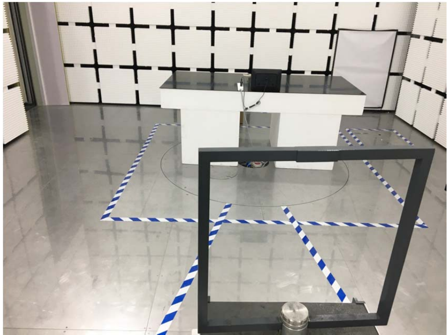
Radiation Emission Test Setup (Below 30MHz)
