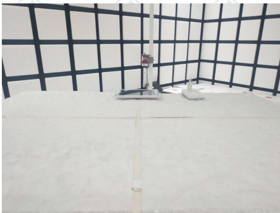
Radiated spurious emission Test Setup-2(Above 1GHz)
