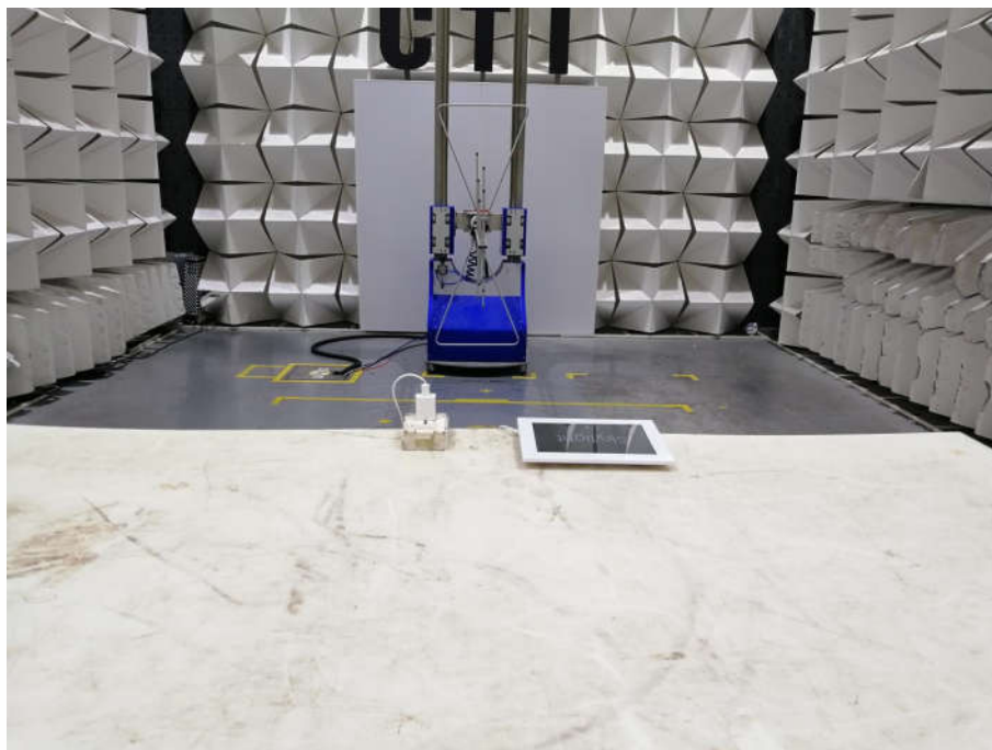
Radiated spurious emission Test Setup-1(Below 1GHz)
