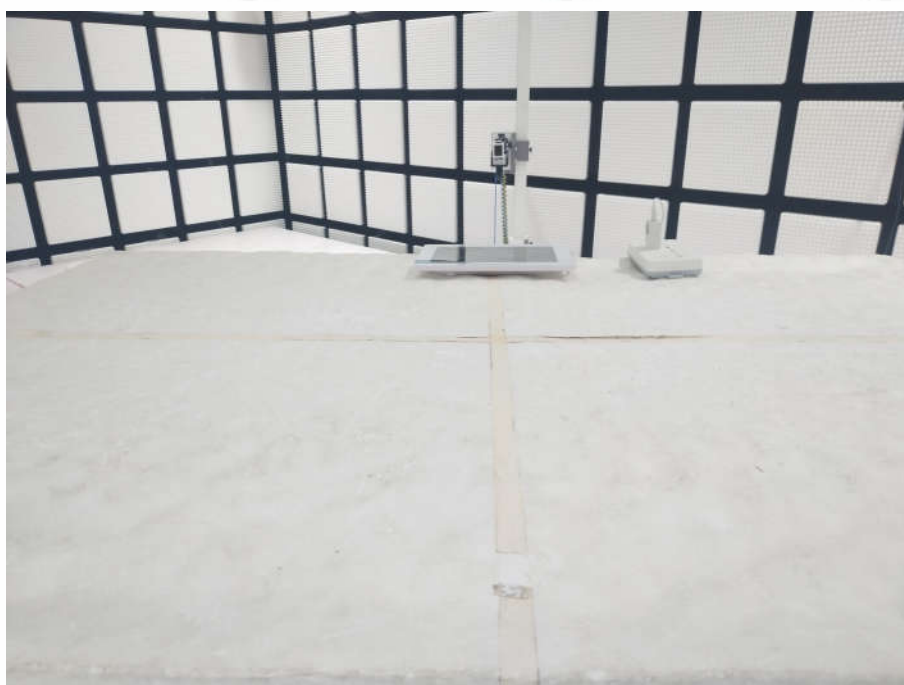
Radiated spurious emission Test Setup-4(Above 18GHz)
