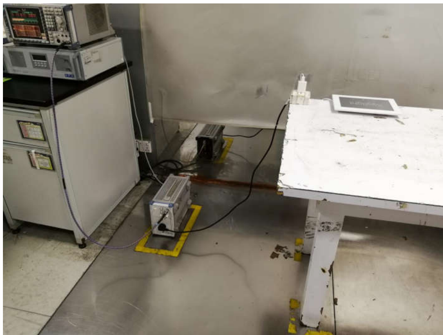
Conducted Emissions Test Setup
