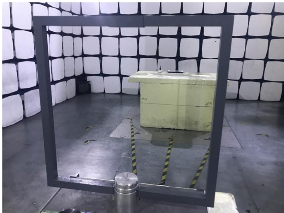
Radiation Emission Test Setup (Below 30MHz)
