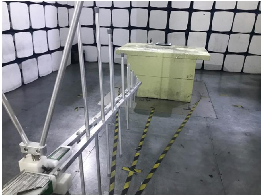
Radiation Emission Test Setup (30MHz to 1GHz)
