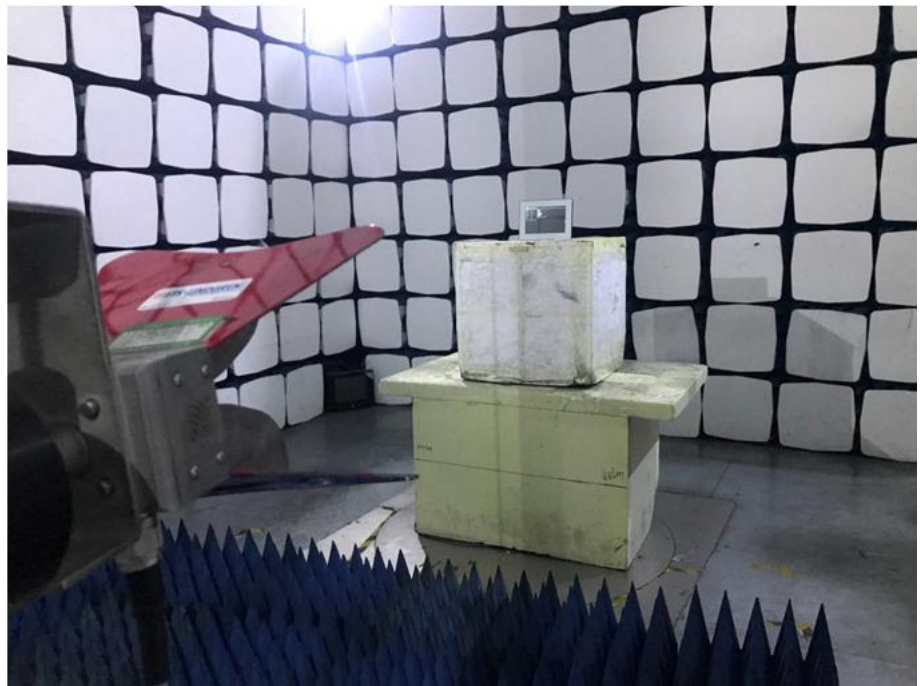
Radiation Emission Test Setup (1GHz to 18GHz)
