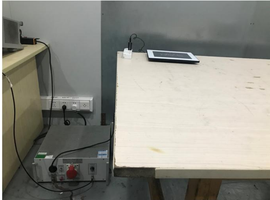
Conducted Emission Test Setup
