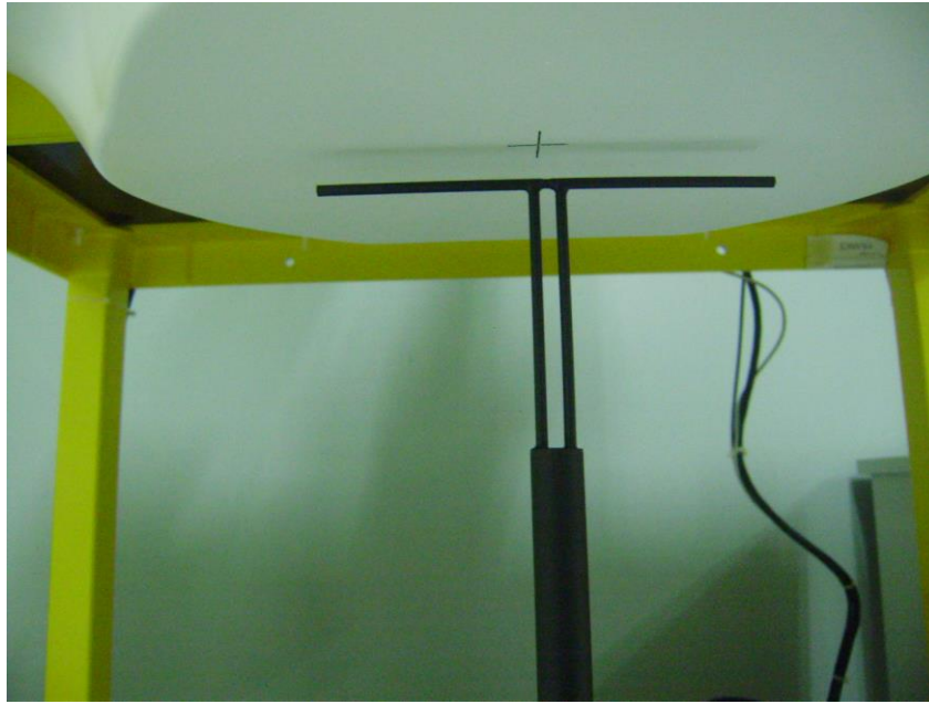
Setup Photo of Dipole Antenna
