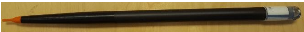
Figure 1 – MVG COMOSAR Dosimetric E field Dipole
