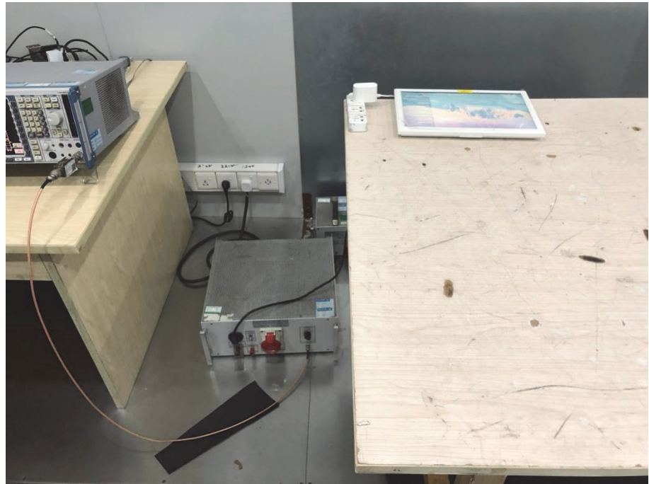
Conducted Emission Test Setup
