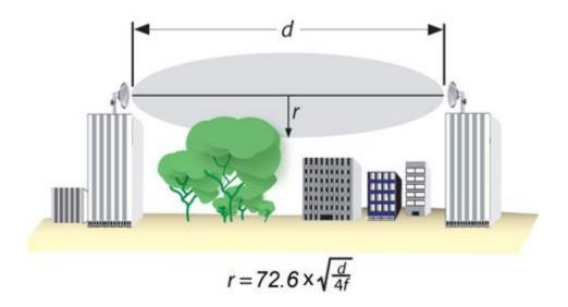
If there are obstacles in the radio path, there may still be a radio link but the quality and strength of the signal will be affected. Calculating the maximum clearance from objects on a path is important as it directly affects the decision on antenna placement and height. It is especially critical for long-distance links, where the radio signal could easily be lost.
