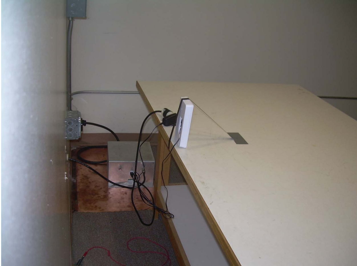
Photograph 4 – Back View Conducted Disturbance Worst Case Configuration
