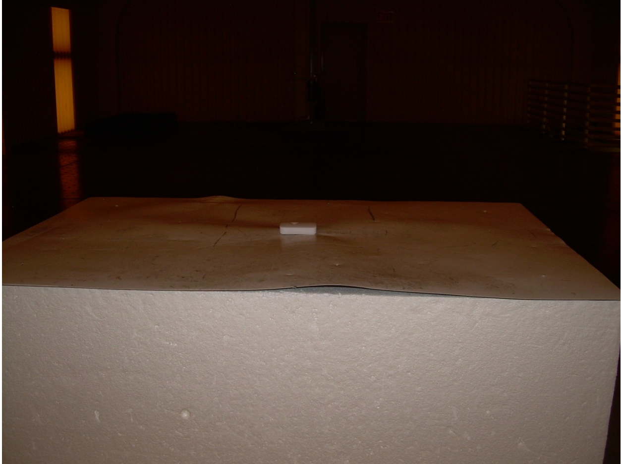
Photograph 2 – Back View Radiated Disturbance Worst Case Configuration – Flat on Table
