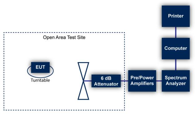
Figure 1: Radiated Emissions Test
