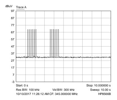
**Graph 2: Plot Showing EUT System Integrity Transmission**
