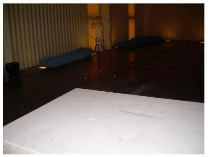
Photograph 5: Test Setup for Emissions Below 30 MHz
