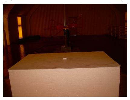
Photograph 2 – Back View Radiated Emissions – 30 MHz to 1000 MHz Configuration
