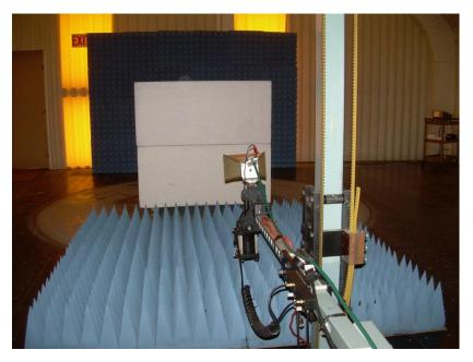
Photograph 7: Test Setup for Emissions Above 1000 MHz
