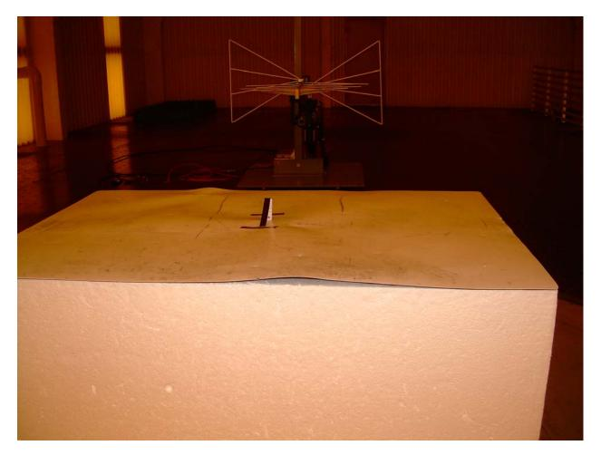
Rear View Radiated Disturbance Configuration – On Edge Placement
