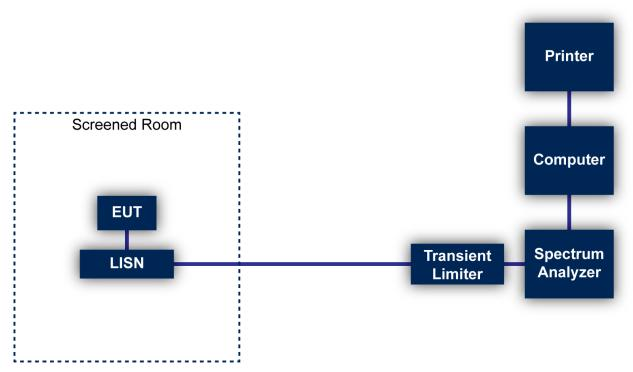
Figure 1: Conducted Emissions Test
