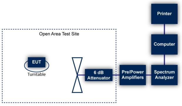
Figure 2: Radiated Emissions Test
