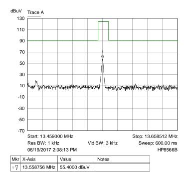
Graph 2: Plot of Fundamental Frequency (Emission Mask Shown)
