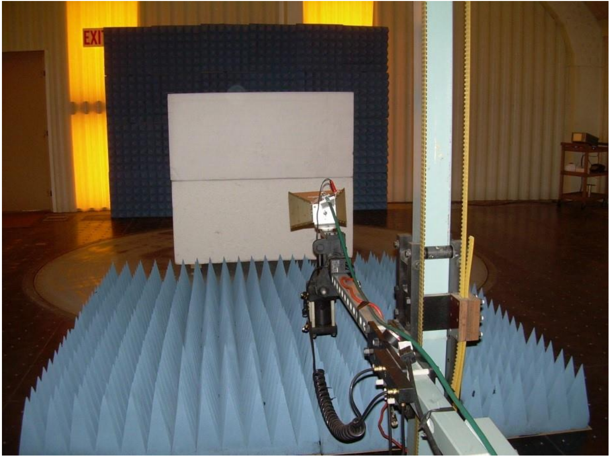
Photograph 9. Test Setup for Emissions Above 1000 MHz
