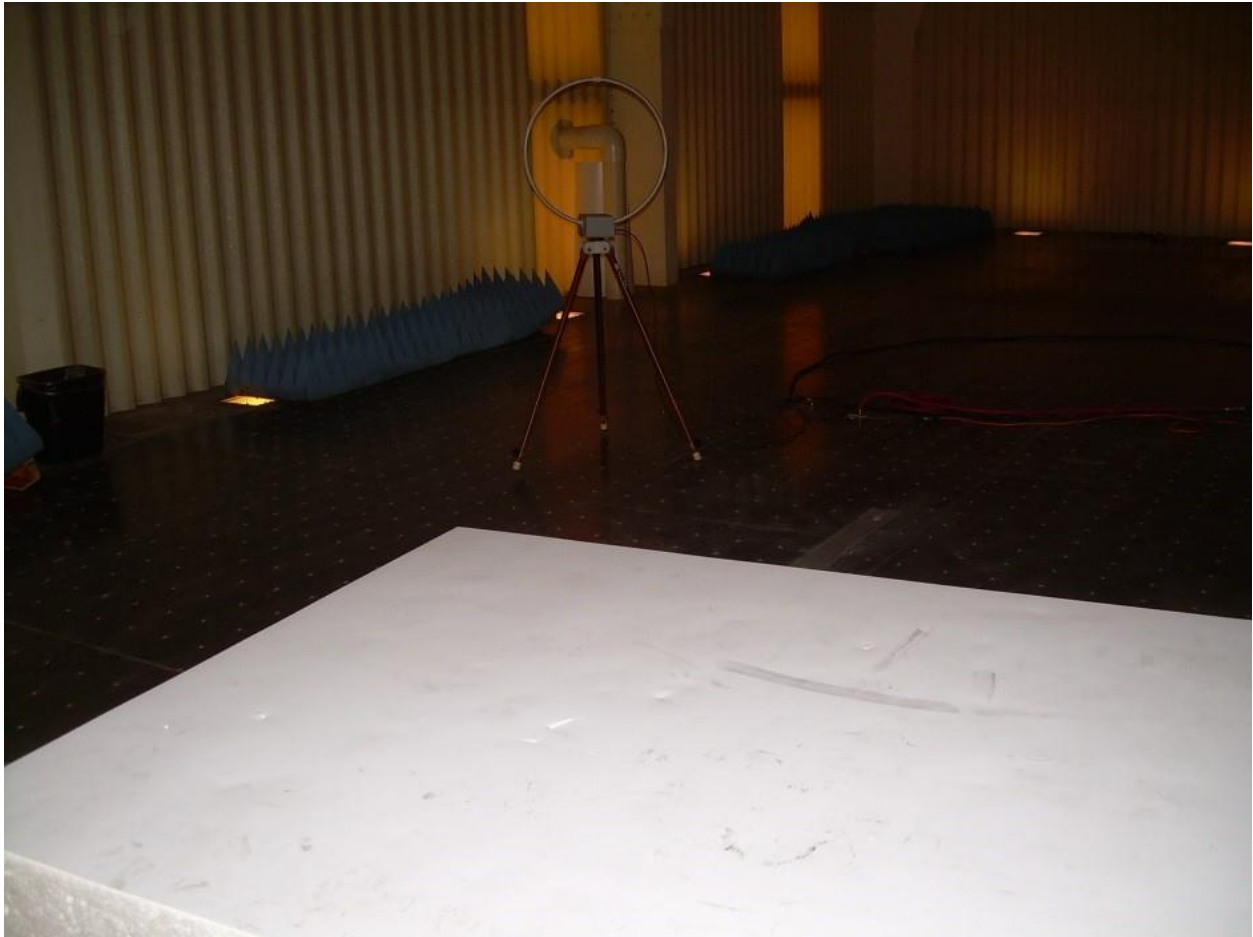
Photograph 7. Test Setup for Emissions Below 30 MHz
