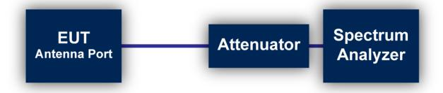
Figure 2: Direct Connection at the Antenna Port Test
