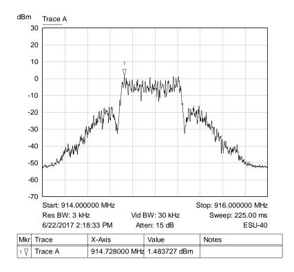
Graph 10: Middle Channel 3 kHz PSD Plot
