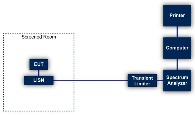
**Figure 1: Conducted Emissions Test**
