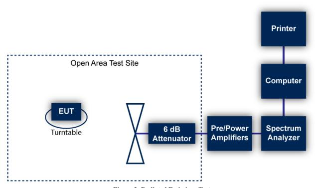
Figure 3: Radiated Emissions Test
