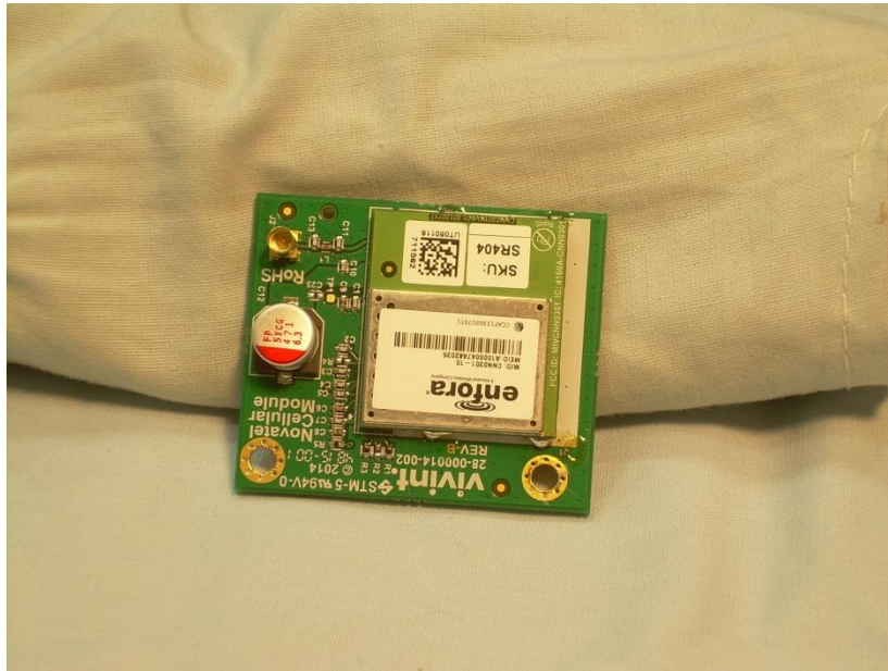
Photograph 20 – View of a Cell Module on the Interface PCB
