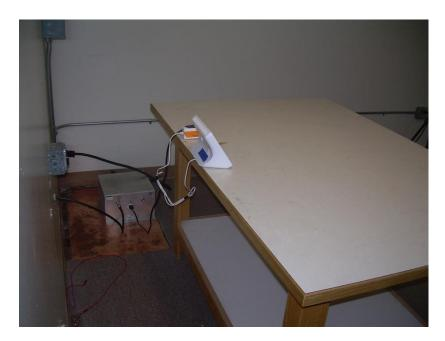
**Photograph 7 - Back View Conducted Emissions Worst Case Configuration**
