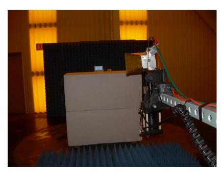
Photograph 3: Front View Radiated Emissions Configuration – Above 1000 MHz
