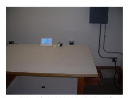
**Photograph 6 - Front View Conducted Emissions Worst Case Configuration**
