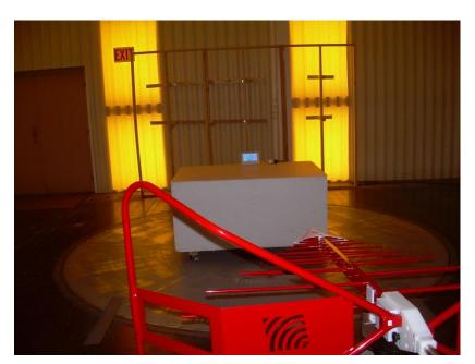
Photograph 1: Front View Radiated Emissions Configuration  $-30-1000\ MHz$
