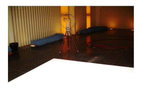
Photograph 5: Loop Antenna Setup Used for Frequencies Below 30 MHz
