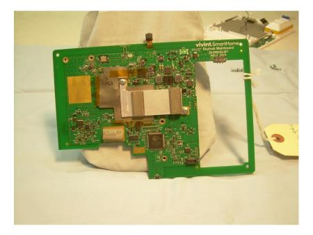
4. Internal View Front Main PCB with Conductive Tape in Place
