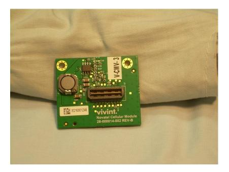
12. View of Already Certified Cell Module Interface PCB
