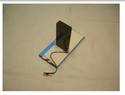
7. Internal View of the Cell Antenna and Battery
