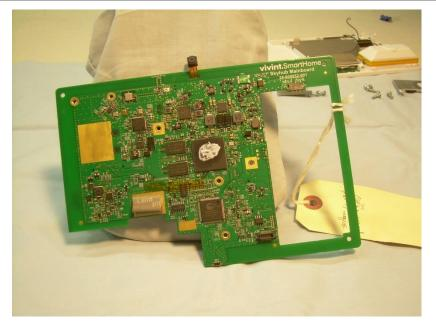
5. Internal View Front Main PCB with Conductive Tape Removed
