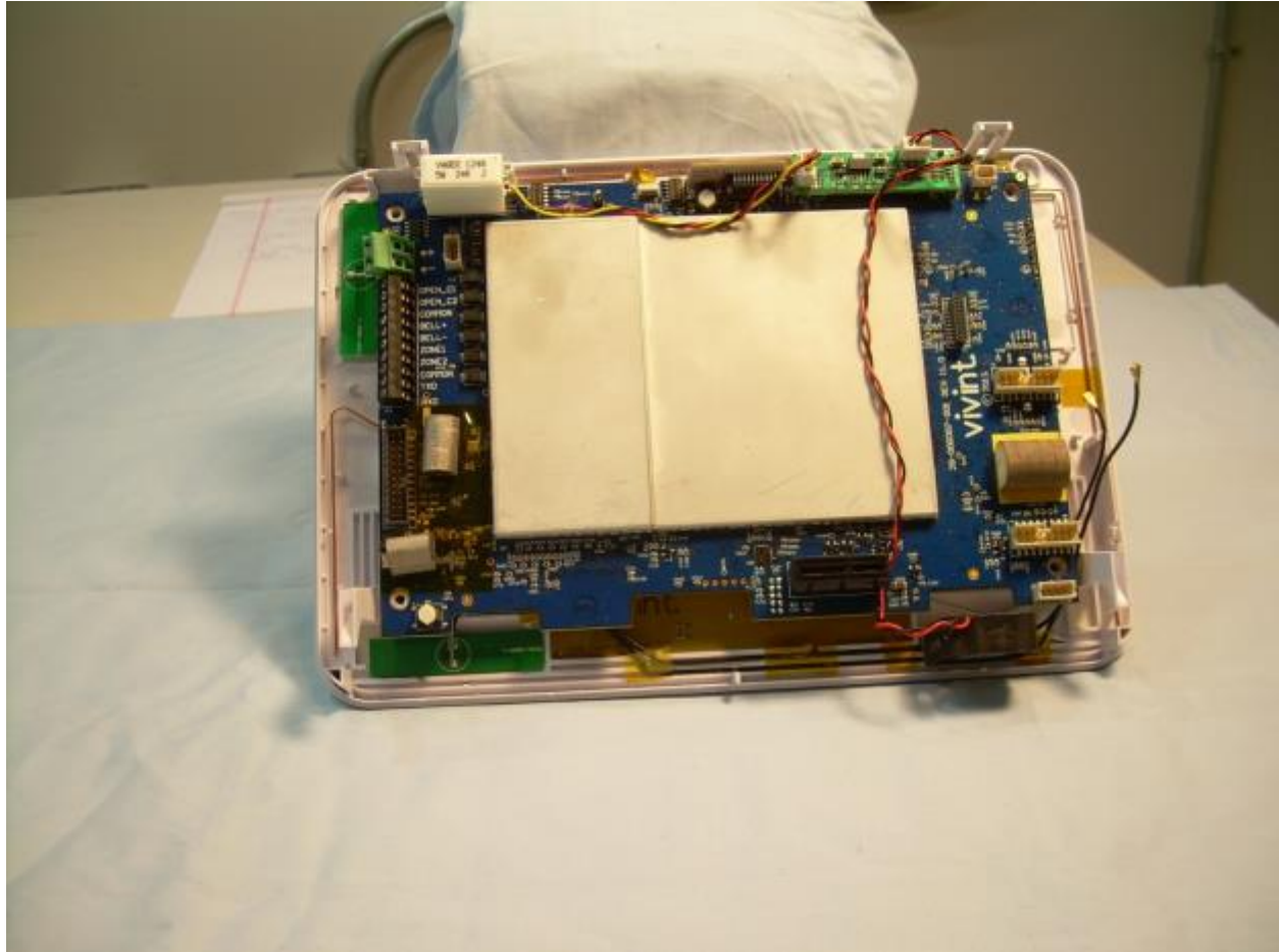
Photograph 12 – View of the EUT with Inner Frame, Hard Drive, and Transceiver Modules Removed
