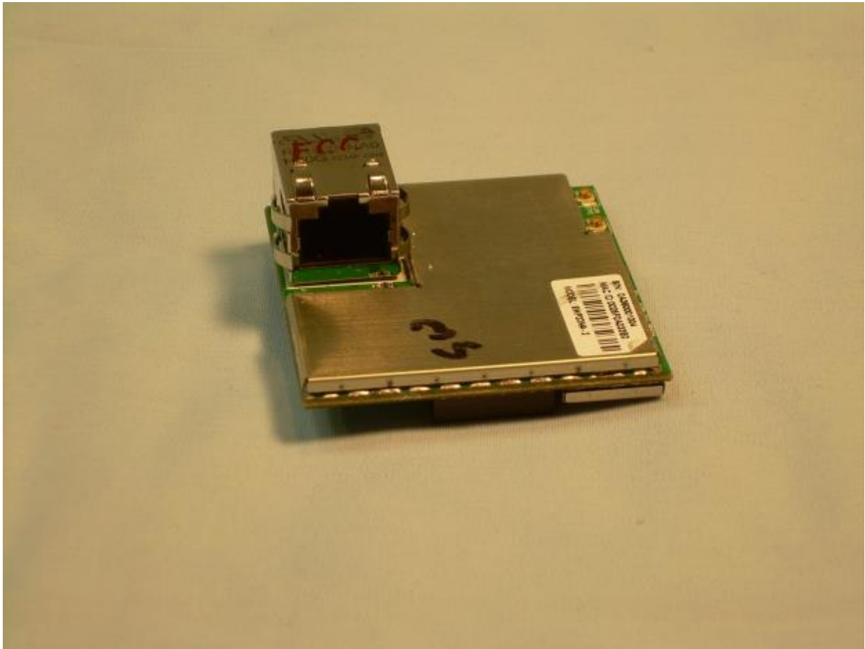
Photograph 21 – View of the Back Side of the Ethernet/WiFi Module
