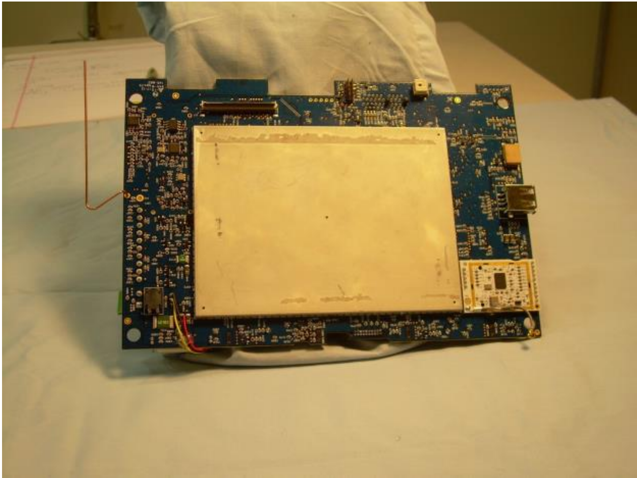
Photograph 14 – View of the Front Side of the Main PCB with RF Shield In Place
