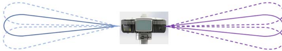
Figure 3: Vertical adjustment of the Pandora360 Radio Lobe.
