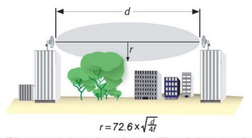
If there are obstacles in the radio path, there may still be a radio link but the quality and strength of the signal would be affected. Calculating the maximum clearance from objects on a path is important as it directly affects the decision on antenna placement and height. It is especially critical for long-distance links, where the radio signal could easily be lost.
