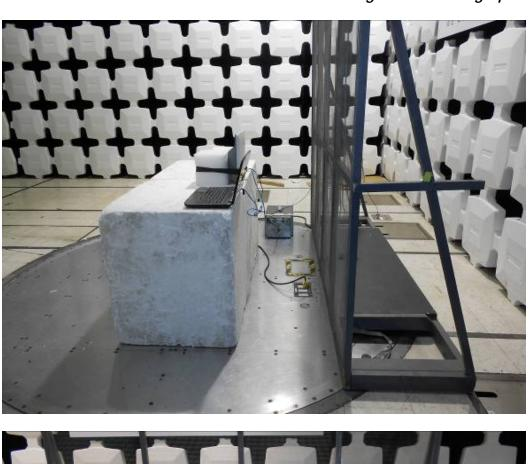
AC Power Line Conducted Emissions Test Configuration Photographs
