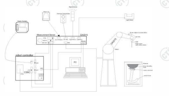
The DASY5 system for performing compliance tests consists of the following items:
