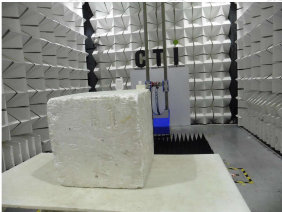
Radiated spurious emission Test Setup for adapter 2(Above 1GHz)
