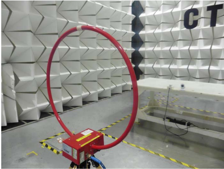
Radiated spurious emission Test Setup for adapter 1(Below 30MHz)
