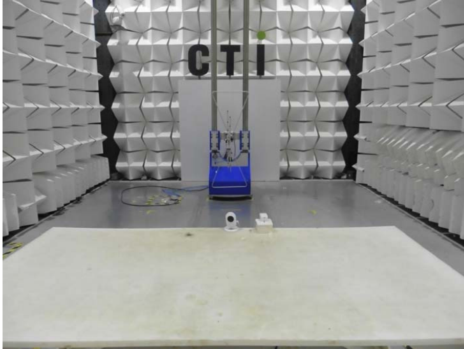
Radiated spurious emission Test Setup for adapter 1(Below 1GHz)
