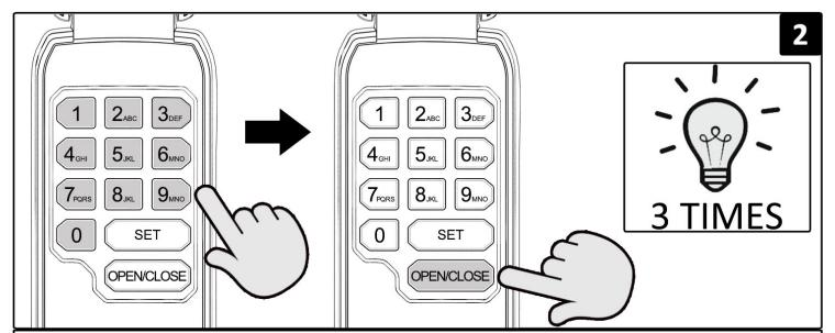
Enter new three to six digit temmporary PIN. Hold the "OPEN/CLOSE" key until motor unit lights blink three times.
