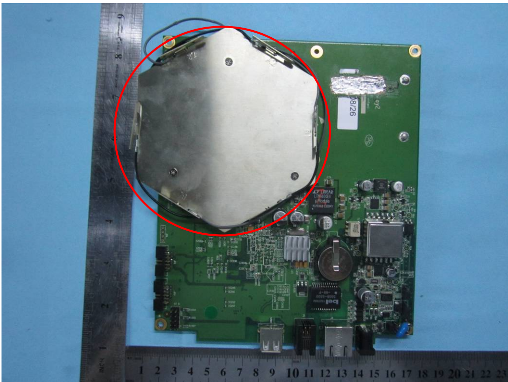
WIFI Antenna View
