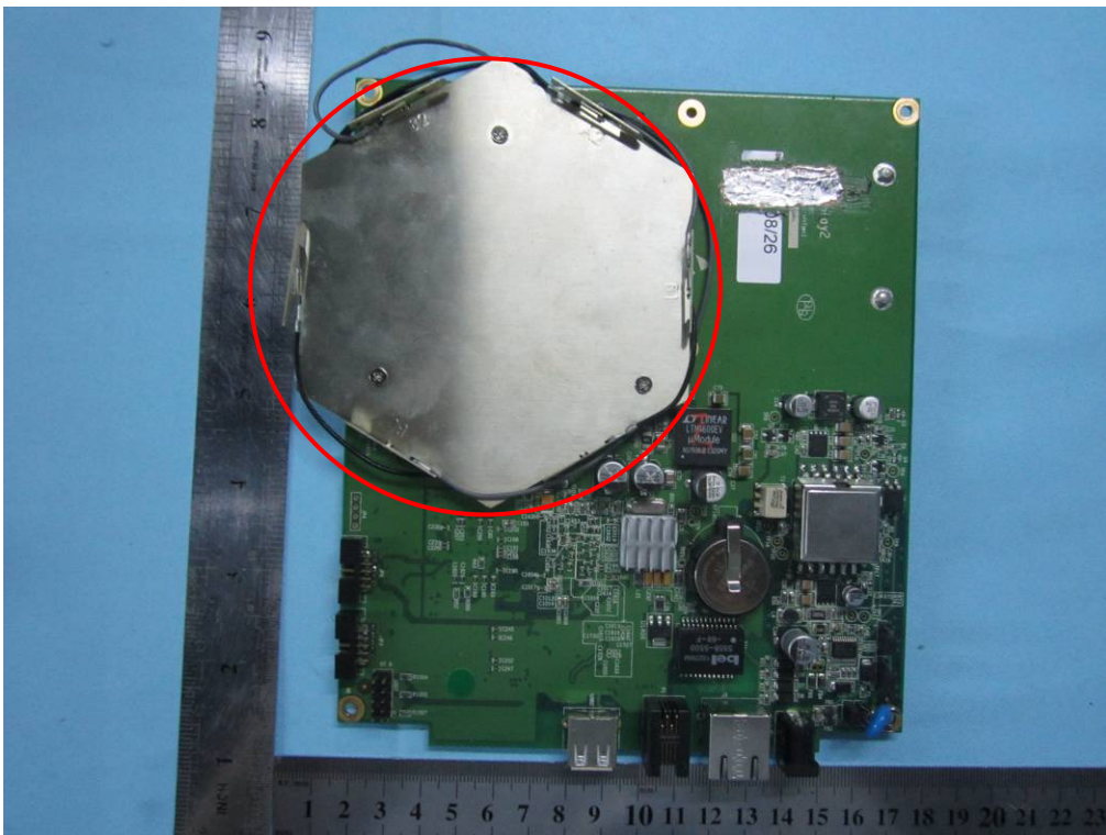
WIFI Antenna View
