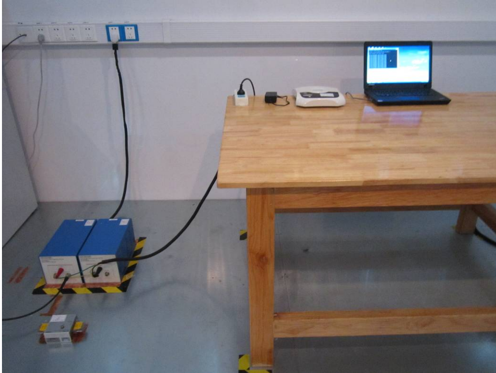
Conducted Emissions Test Setup Front View
