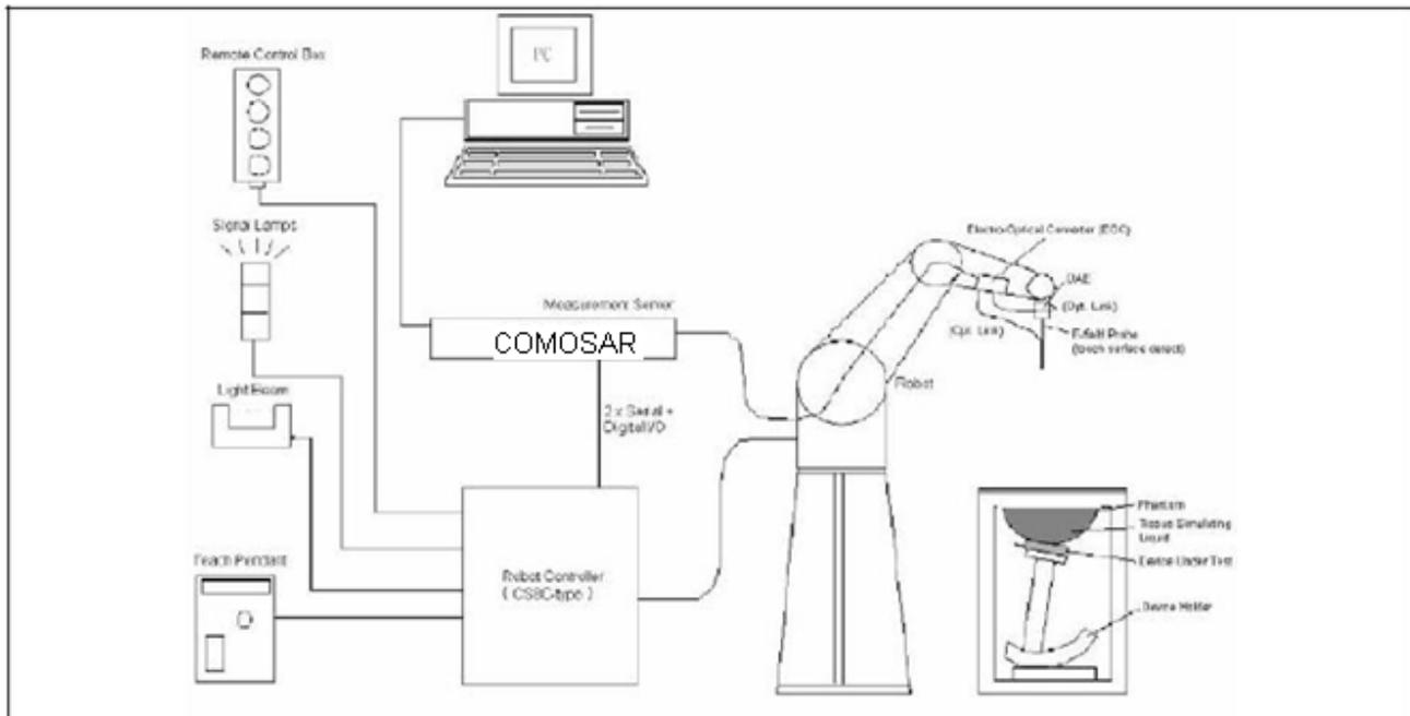
The COMOSAR system for performing compliance tests consists of the following items:
