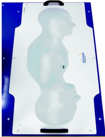
The bottom plate contains three pair of bolts for locking the device holder. The device holder positions are adjusted to the standard measurement positions in the three sections. A white cover is provided to tap the phantom during off-periods to prevent water evaporation and changes in the liquid parameters. On the phantom top, three reference markers are provided to identify the phantom position with respect to the robot.
