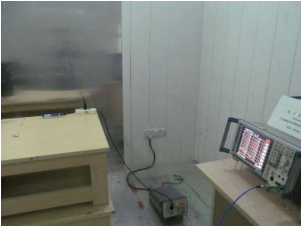
FCC RADIATED EMISSION TEST SETUP
