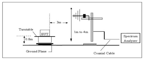
(B) Radiated Emission Test-Up Frequency Above 1GHz
