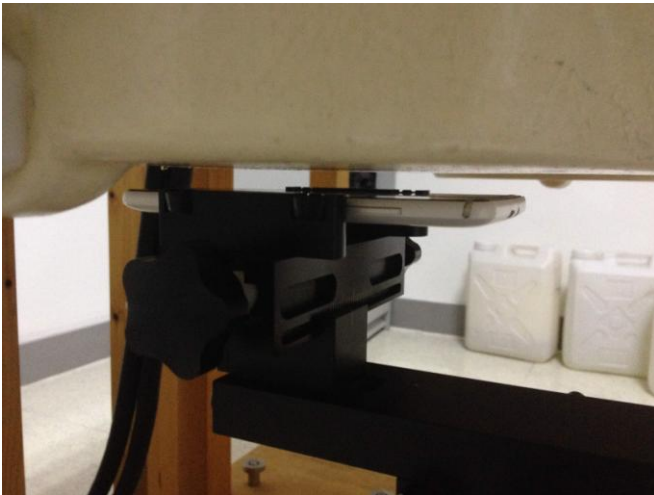
Front of the EUT with 1 cm Gap
