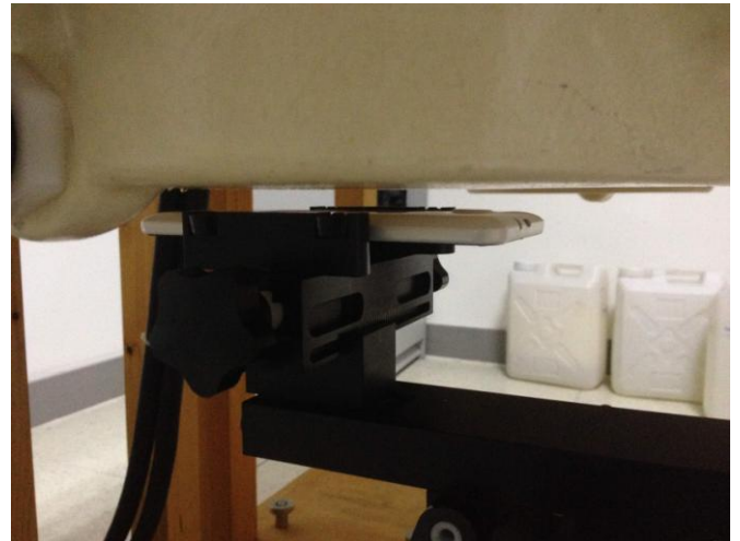
Back of the EUT with 1 cm Gap
