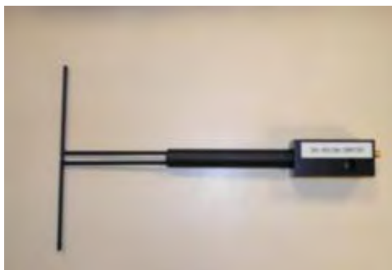
Figure 1 – Satimo COMOSAR Validation Dipole
