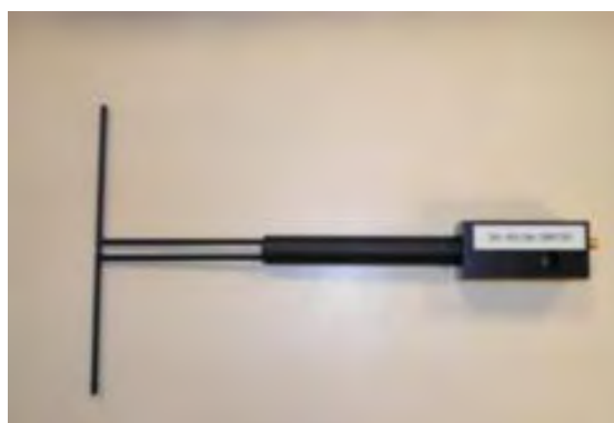
Figure 1 – Satimo COMOSAR Validation Dipole
