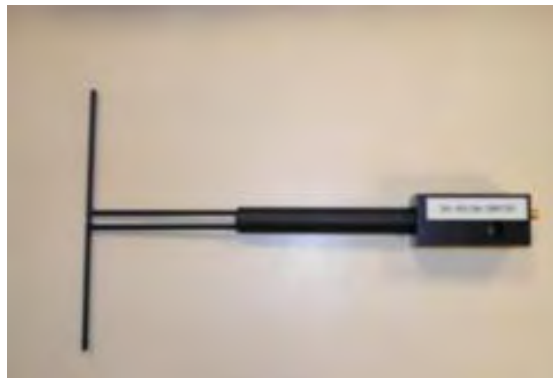
Figure 1 – Satimo COMOSAR Validation Dipole
