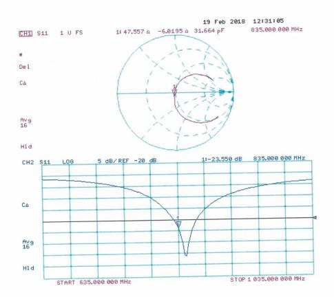
Impedance Measurement Plot for Body TSL
