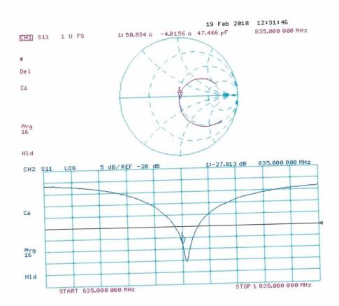
Impedance Measurement Plot for Head TSL
