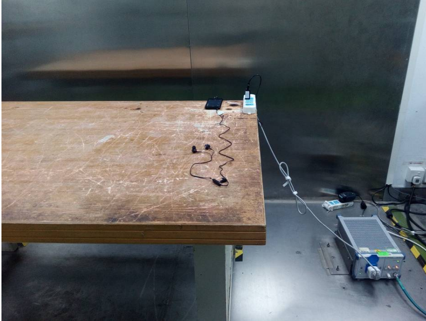
Conducted Emissions - Front View
