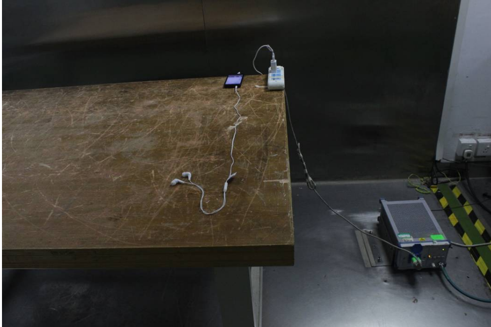
Conducted Emissions - Front View
