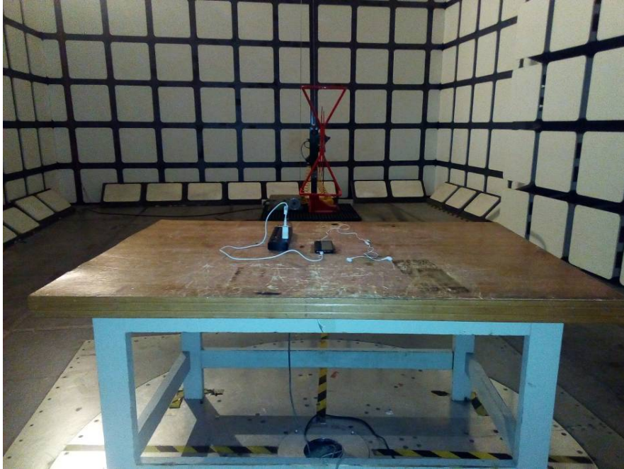
Radiated Emissions View (Below 1 GHz)
