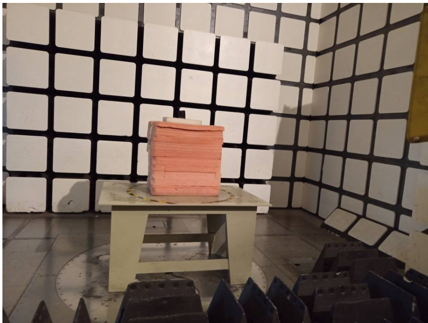
Radiated Emissions View (Above 1 GHz)
