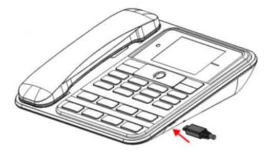
Note: The battery powers the phone for a limited period of time. Make sure the battery is fully charged before using the phone. Make sure that the charger plug and the USB cable plug are inserted in the correct direction. Inserting them in the wrong direction may cause charging failure or other problems. Before charging, make sure that the standard voltage and frequency of the local mains supply match the rated voltage and power of the charger.
