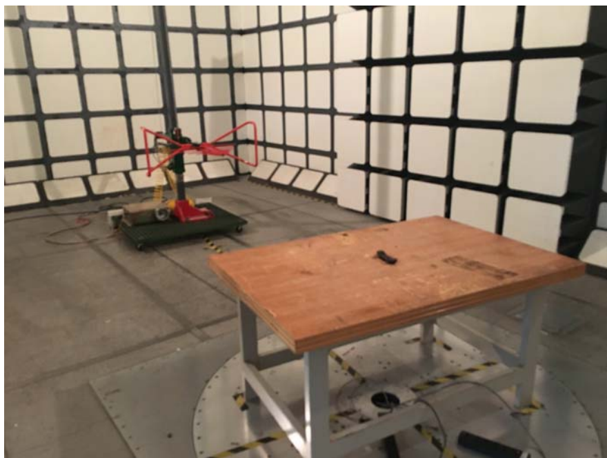
Radiated Emissions View (Below 1 GHz)
