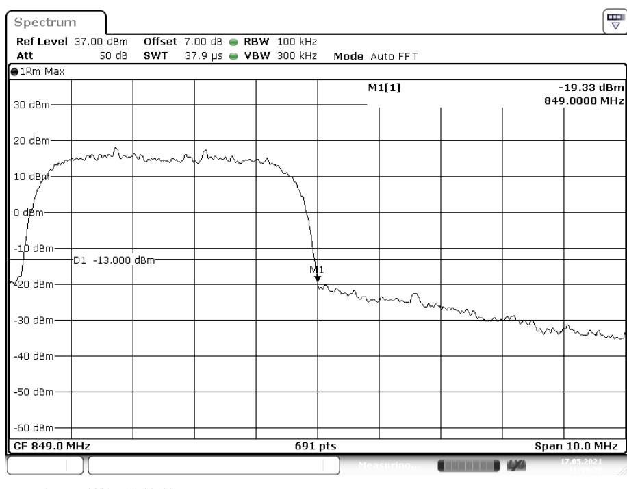
**PCS Band, Left Band Edge for GSM (GMSK) Mode**
