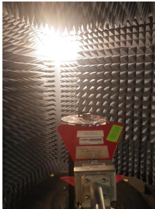
Photograph 2. Radiated Spurious Emissions, Above 1 GHz, Test Setup
