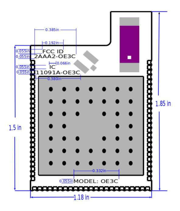
The FCC, IC and model labels will be printed onto the module's PCB board with white silk-screen.
