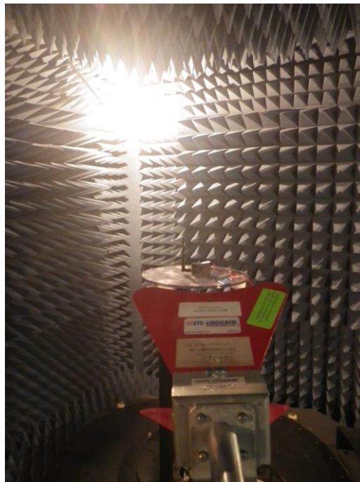
Photograph 3. Radiated Spurious Emissions, Above 1 GHz, Test Setup
