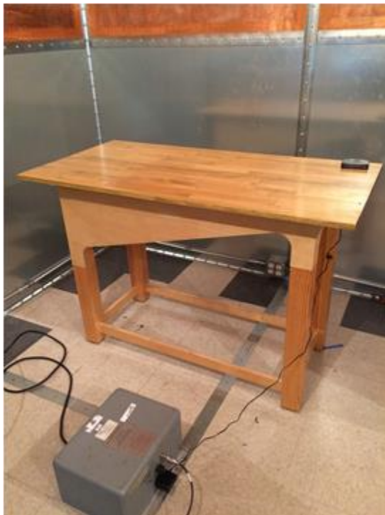
Photograph 1. Conducted Emissions, Test Setup
