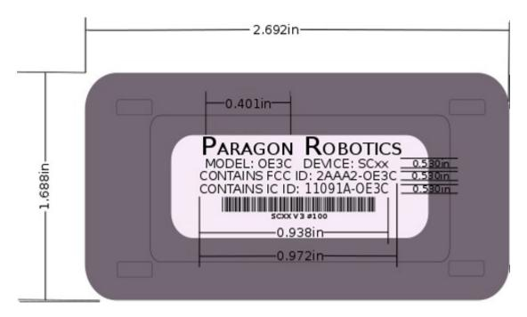
The polymer-based decals are printed using indelible thermal-transfer resin and attached with a permanent adhesive. They are applied on the back of each device case. *Above demonstrates the decal on a sensor case. Below shows the decal on a gateway case.*
