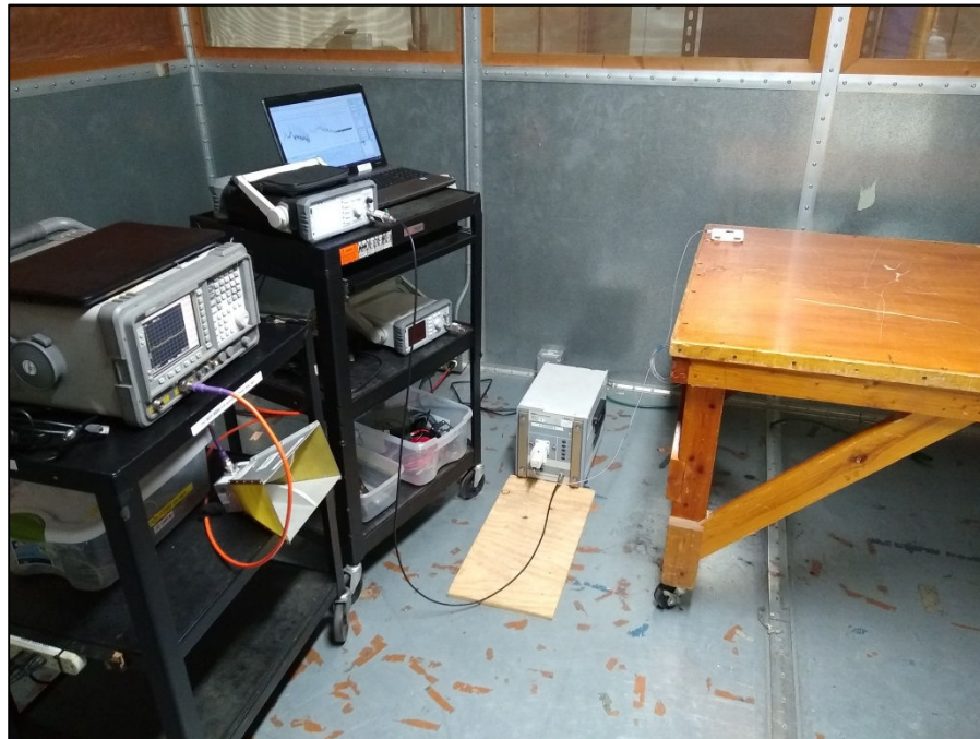
Photograph 3: Conducted Emissions Voltage, Chip Antenna Test Setup
