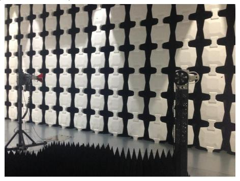
Description: Substitution Antenna for EIRP Test
