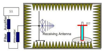
2. The EUT is then put into continuously transmitting mode at its maximum power level during the test. And the maximum value of the receiver should be recorded as (Pr).
