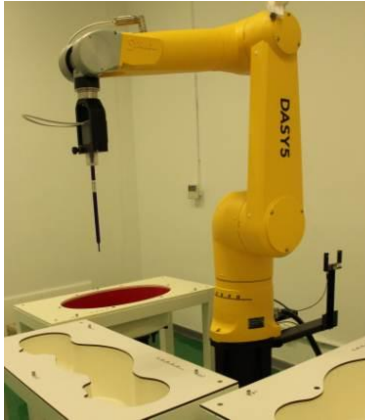
Picture D.6 DSY5 system Set-up
